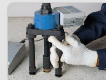
③ Adjust the supporting legs to stabilize the tester.
