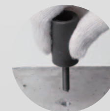
③ Adjust the supporting legs to stabilize the tester.
