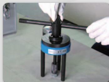
② Screw the coupling into the anchor.
