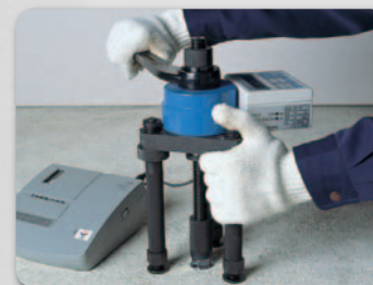
④ Conduct testing by using a box-end wrench to tighten the nut.
